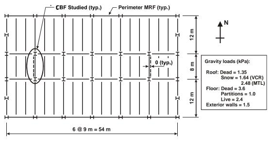
Figure 1: Plan view of the studied building and design gravity loads
