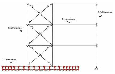
Figure 3. OpenSEES model of structure-foundation-soil system (adapted from Aguero (2006) and Prishati (2008)).
