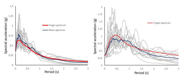
Figure 3. Target acceleration spectrum, individual record spectra and mean 5% damped elastic acceleration spectrum for calibrated ground motions: (a) MTL-E and (b) VCR-E.
